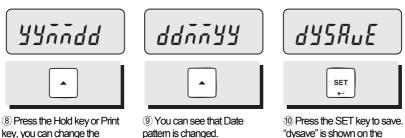
10 Press the SET key to save. "dysave" is shown on the display shows a day of the week. If you set up a day of the week wrong, "dy err" is shown on the display.
