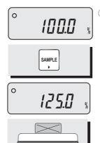
③ Place reference sample on the platter and press the SAMPLE key. The display shows "100.0". Make sure that reference sample bigger than 3% of maximum capacity. If it is lower than 3% of maximum capacity, the display shows "tow". In this case, increase the weight of reference sample and press the SAMPLE key.
